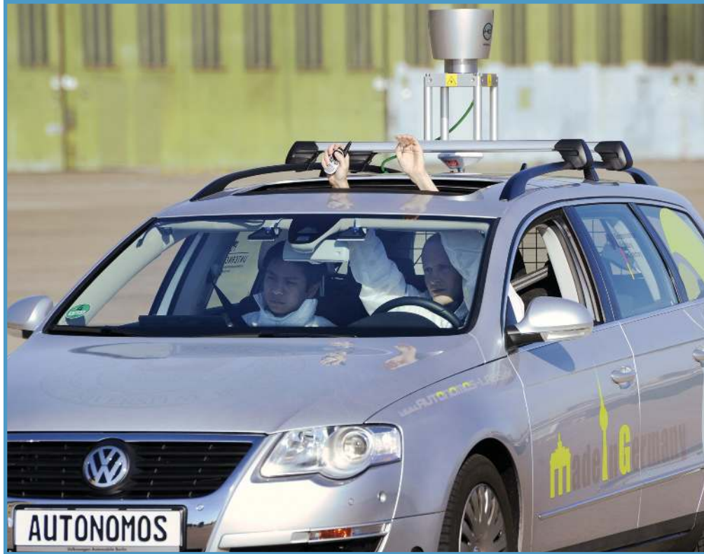
Figure 5.3 In October 2010, German engineers at Berlin’s Free University unveiled the latest self-driving car, which proponents say will sharply reduce accidents, help the environment, and transform cities. The car is called “Made in Germany,” or MIG, for short. Although it looks like an average Volkswagen Passat with a camera on top, MIG uses cameras, laser scanners, and satellite navigation to “see” other vehicles and pedestrians and deal with traffic situations.
